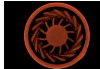
Sintered micro turbine ( \varnothing 3 \text{ mm} )
